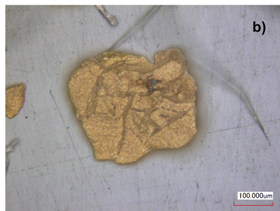
Fig. 8. (a) Thermogravimetric curves of Au(III)-loaded CAF, and the original CAF; (b) confocal microscope image of Au(III)-loaded CAF after incineration.
